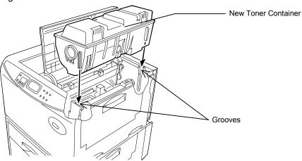
**9.** Check that the toner container is installed in the correct position, and push forcefully on the top of the toner container as shown in the figure.
